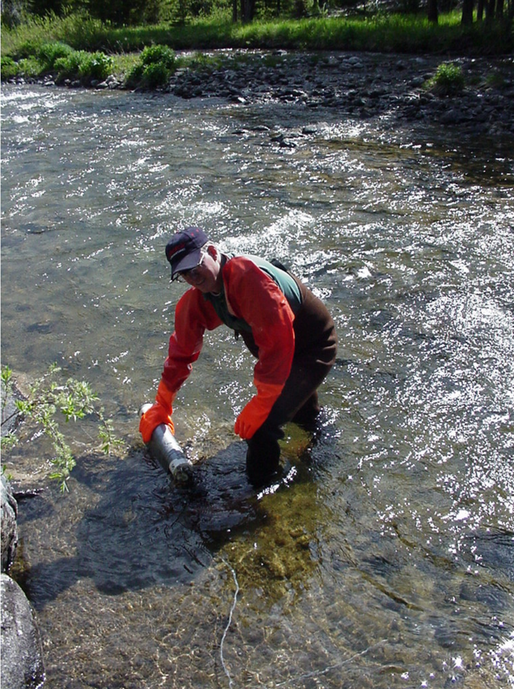
Photograph 2. Location of the Hydrolab for measuring turbidity downstream of the powerhouse discharge. Photograph taken on June 15, 2005.
