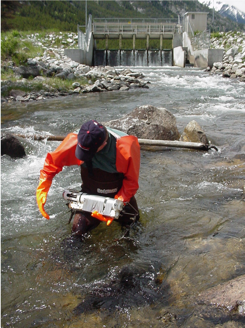
Photograph 1. Location of the Hydrolab for measuring turbidity downstream of the re-regulation dam. Photograph taken on June 15, 2005.
